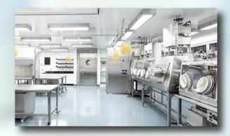
Containment laboratories require air pressure negative to atmosphere to stop the escape of hazardous pathogens, which is achieved by the specialist airflow created by the HVAC system and room design.
