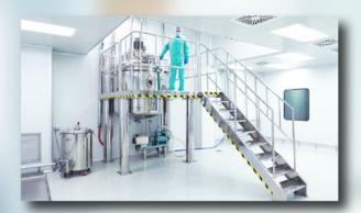
Cleanrooms maintain positive pressure to protect the product. This is achieved by specialist airflow created by the HVAC system and room design. They are used in many sectors, such as electronics, research and pharmaceutical manufacturing.
